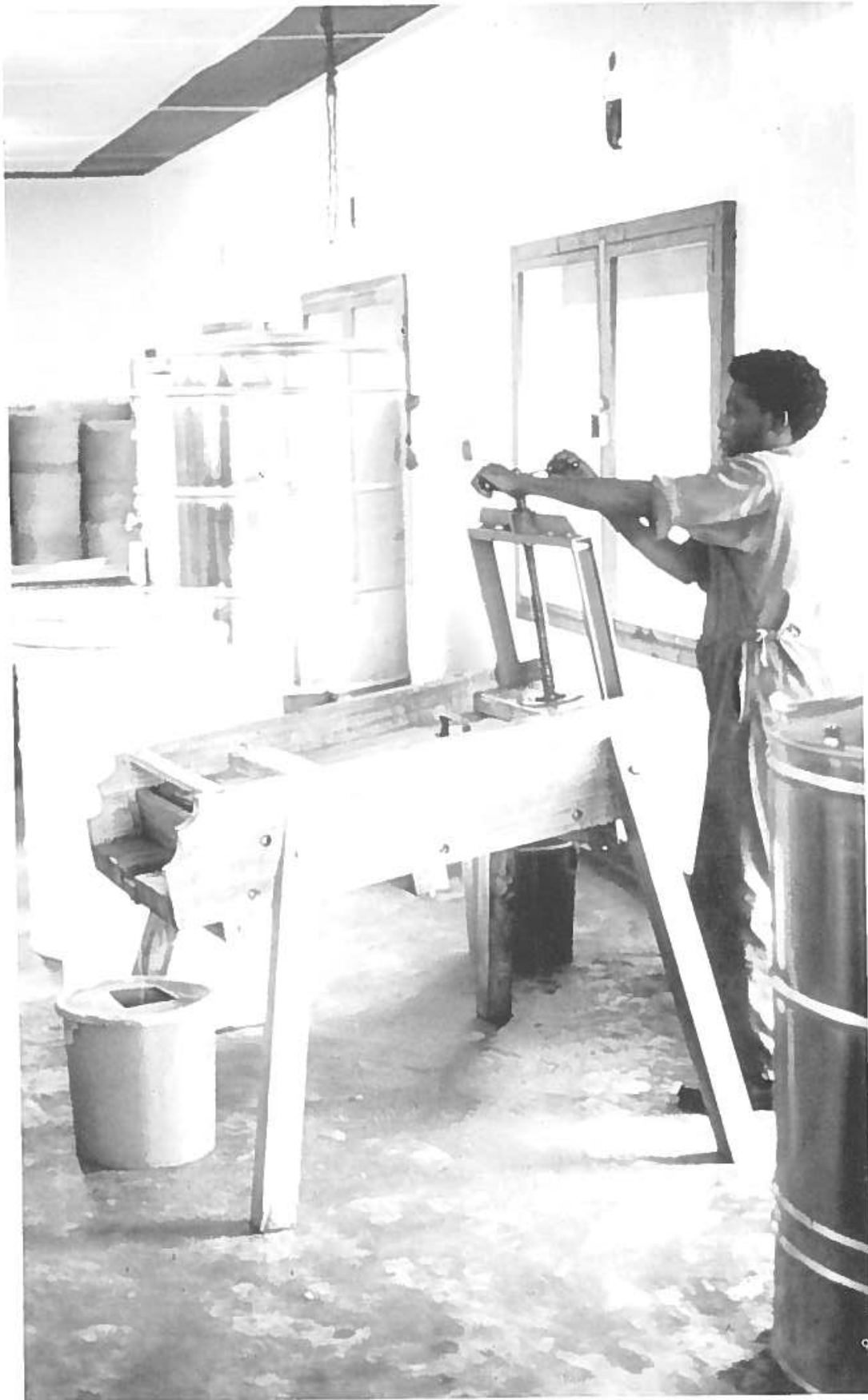
Figure 4. Pressing the honey combs in the factory
